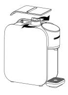
Remove the top cover and install the DF-C combined cartridge into the main body.
